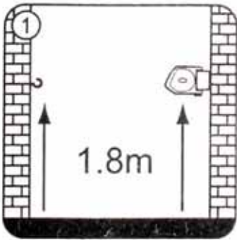
1 Select Wall Positions. (Approx 1.8m above the ground level)
